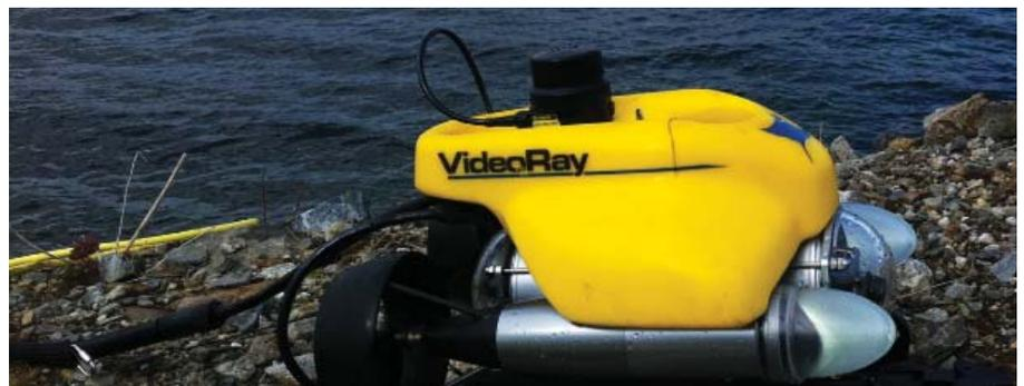
VideoRay Pro4 ROV with Tritech sonar and positioning system
